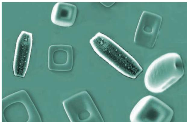
resolution than CFL. A unique feature of the new method is that the particles formed are not just spherical – it can make a wide range of shapes. SFL also allows the formation of particles in biocompatible and easily functionalised materials that are not typically amenable to
