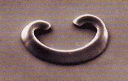
A new microfluidic polymer "printer" can cheaply make 50-micrometer fluorescing bar-coded particles (left) or custom shapes (top and bottom) for other applications.
