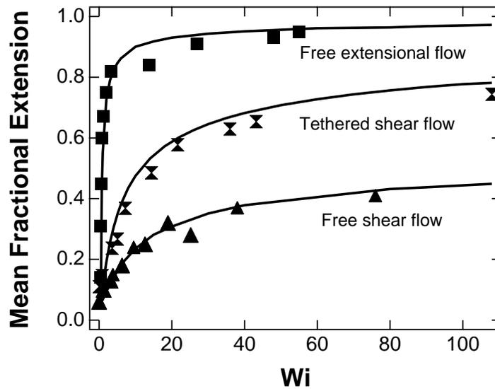
Figure 2: Comparison of Brownian dynamics simulations (lines) to single molecule DNA experiments (symbols). Mean fractional extension (stretch of the DNA scaled by the contour length of the molecule) versus Weissenberg number ( $Wi$ ) is shown for tethered and free DNA in linear hydrodynamic flows. The  $Wi$  is the product of the shear rate (or elongation rate) and the longest relaxation time of the DNA. Figure adapted from Doyle et al. (2000).
