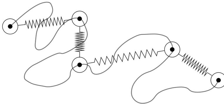
Figure 1: Schematic of the canonical polymer model used in Brownian dynamics simulations: a bead-spring chain. The continuous curve is the 'real' polymer that the bead-spring chain is meant to represent.
